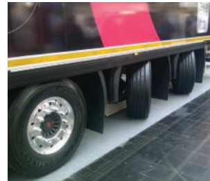
VSE's dual command steer system significantly reduces tyre scrub
